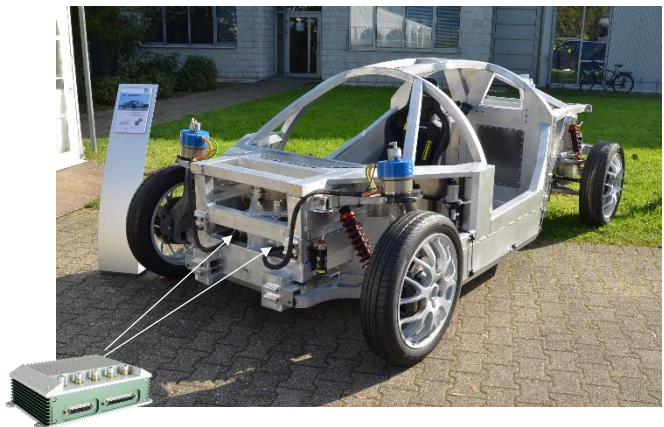
SpeedE with Integrated Steer-by-Wire System
